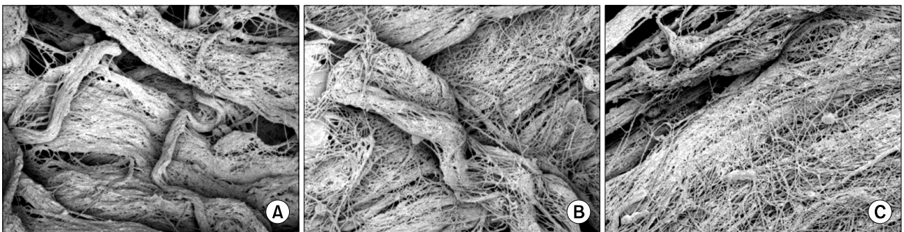
Fig. 6. Electron microscopic findings (after the fatigue test). (A) Glutaraldehyde fixation only; (B) glutaraldehyde fixation+decellularization; (C) glutaraldehyde fixation+decellularization+ \alpha -galactosidase. Interstitial derrangement was observed in B and C. C had more deranged interstitium than B ( \times 3,000 ).
